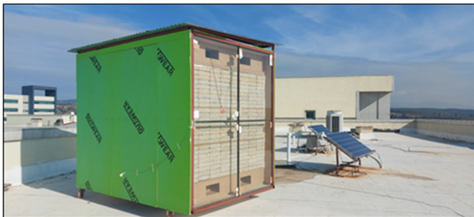
Fig. 4. Test system of Composite Trombe Wall [17]
